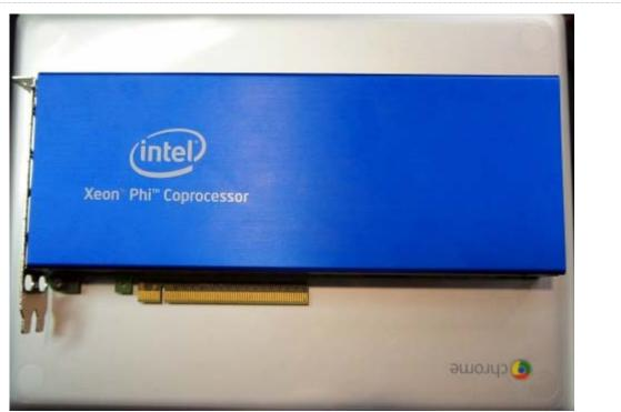
Intel this week released its new high-performance chip, its Xeon Phi co-processor, a 60-core chip that can deliver up to a teraflop of performance. To give you an idea of its size, it is shown here sitting on a Chomebook Samsung 5 550, 12.1-inch model which uses an Intel Celeron processor. The latest Samsung Chromebook model uses the Samsung Exynos ARM processor that the Barcelona Supercomputing Center is deploying in its supercomputer.
