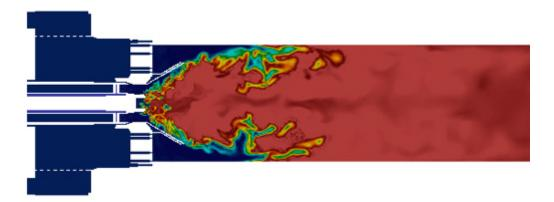
The design of modern combustion systems needs to address challenges related to reduction of pollutant emissions, flexibility of operation while avoiding thermo-acoustic instabilities. The use numerical simulations is important as they provide detailed insights into the performance of the systems.
