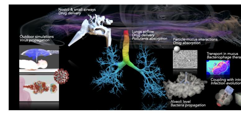
The project aims at predicting particle deposition in the respiratory system, drug delivery being the main target application. To this end, direct numerical simulation of the airflow and Lagrangian particle transport are carried out in the large and small airways.
