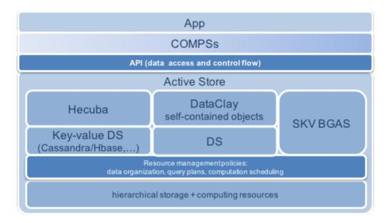
The Storage API can be implemented by multiple Storage Backends. The Storage Backend is responsible for storing data in a set of distributed resources, managing data format and organisation and optimising data queries. Currently, the Storage API does not provide any functions to manage transactions, so the consistency guarantees offered to applications are inherited from the Storage Backend used.
