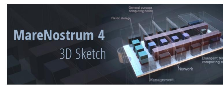
The new supercomputer will have a performance capacity of 13.7 Petaflop/s and so will be able to carry out 13,677 trillion operations per second.
