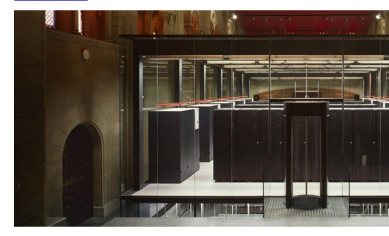
**MareNostrum** was a supercomputer of the BSC-CNS based on PowerPC processors, the architecture BladeCenter, a Linux system and a Myrinet interconnection. These four technologies configure the base of the architecture and design.
