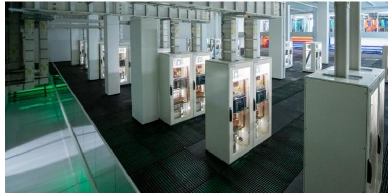
MareNostrum 5 is a pre-exascale EuroHPC supercomputer hosted at BSC-CNS. The system is supplied by Bull SAS combining Bull Sequana XH3000 and Lenovo ThinkSystem architectures and it has a total peak computational power of 314PFlops. The system will provide 4 partitions with different technical characteristics that jointly can fulfill the requirements of any HPC user.
