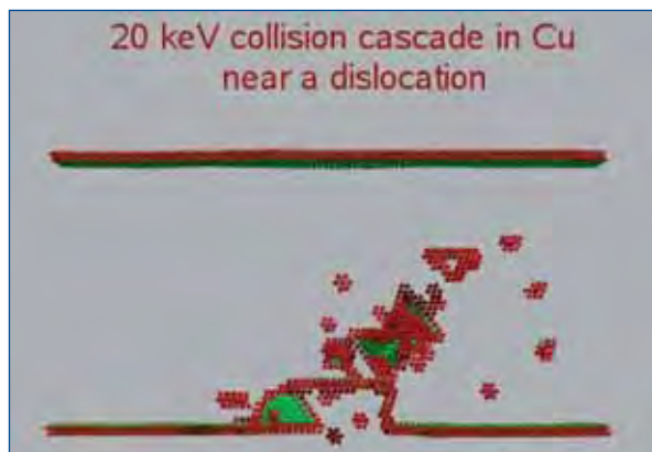
Calculations of collision cascades next to dislocations in Cu.
